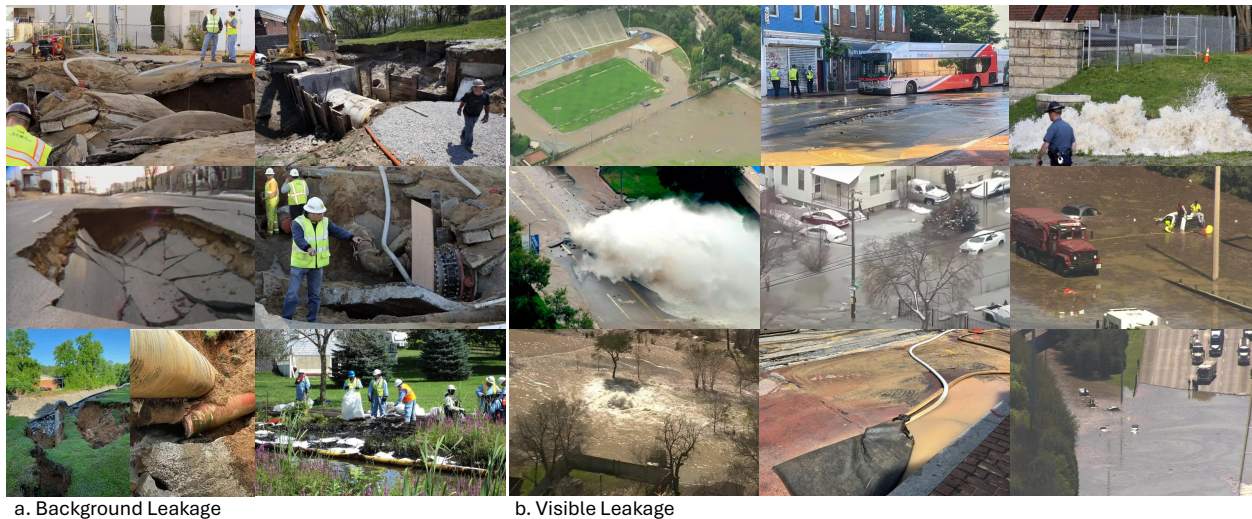
Figure 1: Critical pipeline infrastructure failures demonstrating the urgent need for automated monitoring systems. (a) Background Leakage: The silent majority of pipeline failures occur as gradual, undetected leaks that persist for months or years. These images show typical background leakage scenarios including subsurface water accumulation, soil erosion, corroded pipe segments, and contaminated groundwater infiltration. Such leaks waste millions of gallons of clean water annually and allow untreated sewage to contaminate soil and groundwater, often going unnoticed until environmental damage becomes irreversible. (b) Visible Leakage: Catastrophic failures that disrupt urban life, resulting from either sudden mechanical damage (construction accidents, ground movement) or progressive deterioration from undetected background leaks that escalate to structural collapse.
